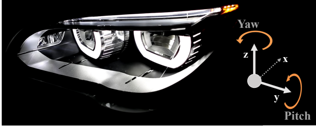
Fig. 2: Visualization of Yaw and Pitch rotation DoFs of the headlight
